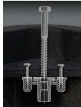
Non-Seizing Bolt System Allows Field Replacement
